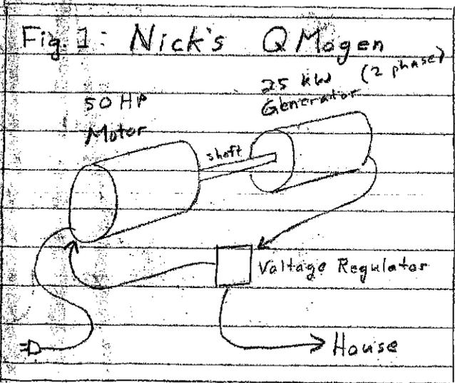
In figure 1 to the right is a simplified representation of the QMagen that Nick's dad pulled together. The 50 HP motor would be plugged into the grid to bring the system up to speed, at which point they would unplug it and it would remain in operation, being powered from the voltage regulator. Nick said that wire was spliced into the wire coming from the plug. The shaft coming from the motor was attached to the 25
